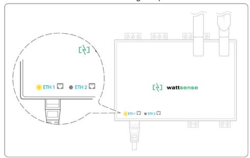
Connect all equipment to the switch via the Ethernet cables.
