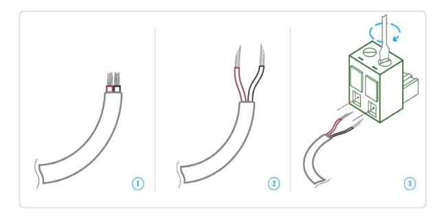
Connect the cable to the power supply.
