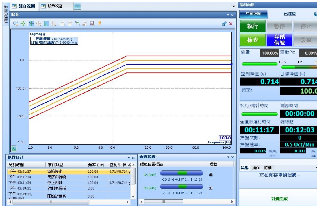
Y Axis resonance sweep - G-sensor
