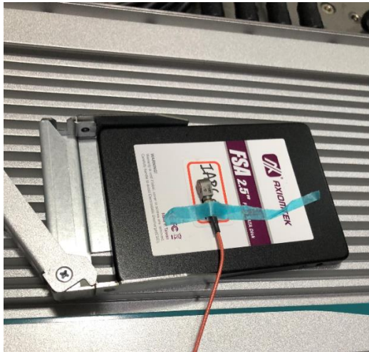
X Axis resonance sweep - G-sensor
