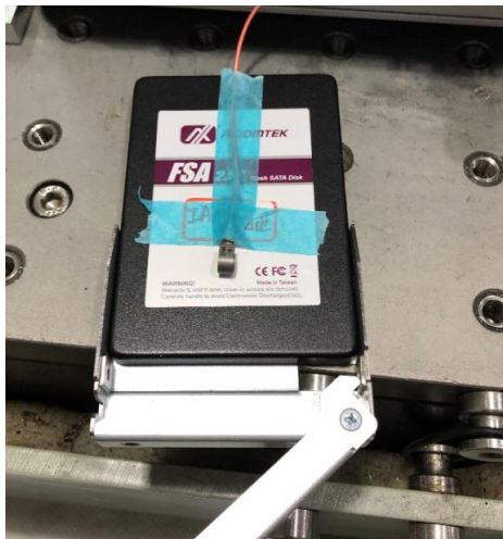
Y Axis resonance sweep - G-sensor
