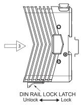
and push the DIN rail lock latch to the latched (in) position.
