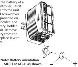
To maintain UL rating, battery must be replaced with one listed in the Specifications.
