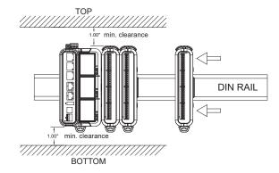
Figure 1 - Attach modules to Controller on DIN Rail
