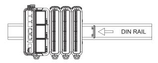
Figure 2 - Attach dust cap to last module
