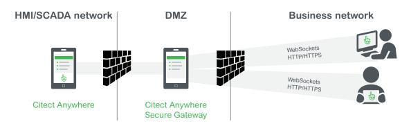
Citect Anywhere Secure Gateway is a complimentary component of Citect Anywhere that provides remote access to Citect SCADA clients.
