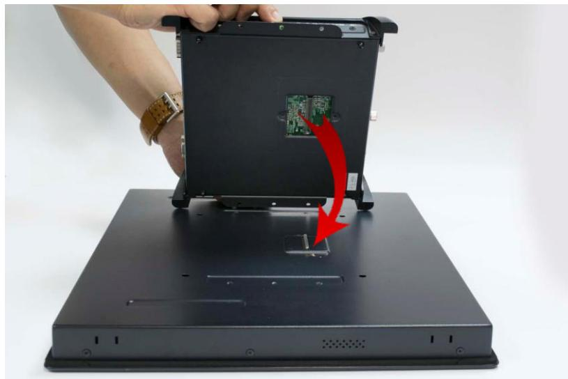
2. Press the PC module downward to ensure two modules are firmly connected.
