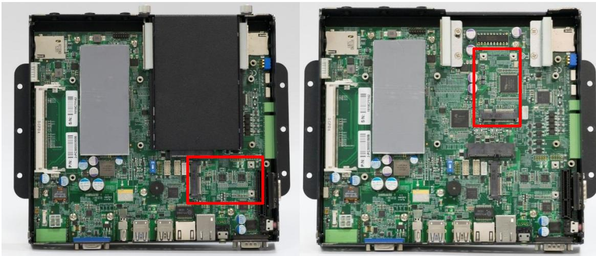
2. Insert mini PCIe card or mSATA module from 45 degree direction.
