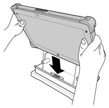
Using one hand, carefully push the top of the R11AH Tablet PC backward until the latch is fully
