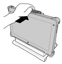
Ensure the R11AH Tablet PC is tightly secured to the docking cradle.
