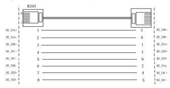
MDI/MDI-X auto connection makes switch easy to use for customers without considering the type of network cable.
