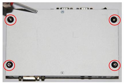
**Step 3** Fix the VESA mount to the correct location, and fasten all screws.
