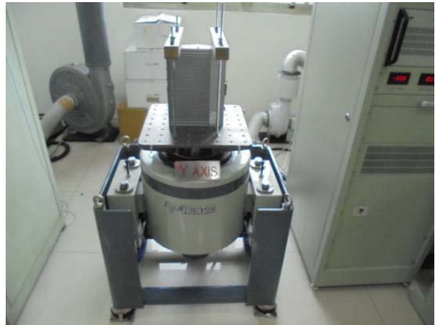
FIG.3.4 : Y Axis direction mounted.
