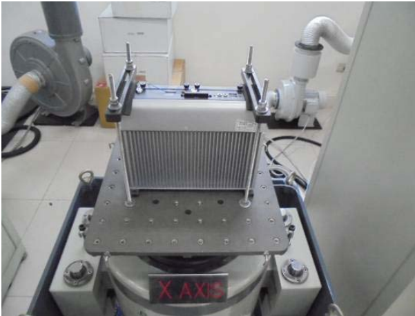
FIG.1.1 : X Axis direction mounted.
