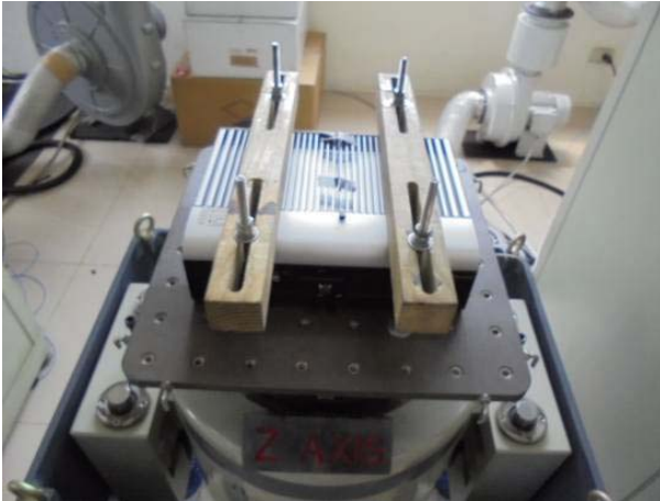
FIG.5.1 : Z Axis direction mounted.
