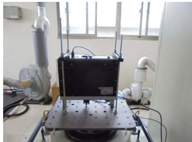
FIG.7.4 : X Axis direction mounted.
