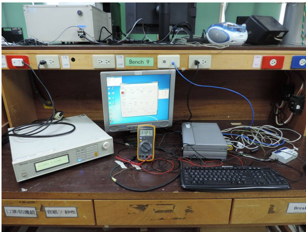
Supply variations Test(Test Voltage:31.2VDC)
