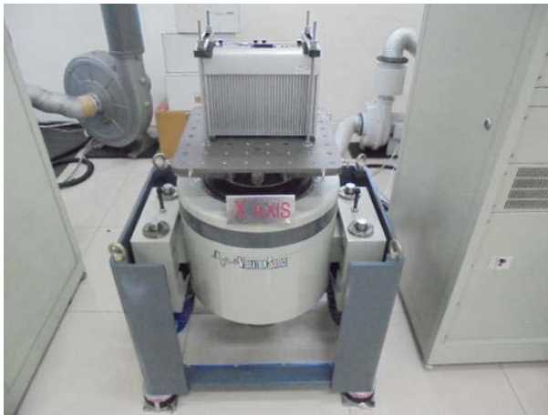
FIG.1.3 : X Axis direction mounted.
