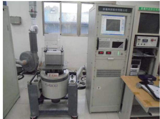
FIG.1.4 : X Axis direction mounted.
