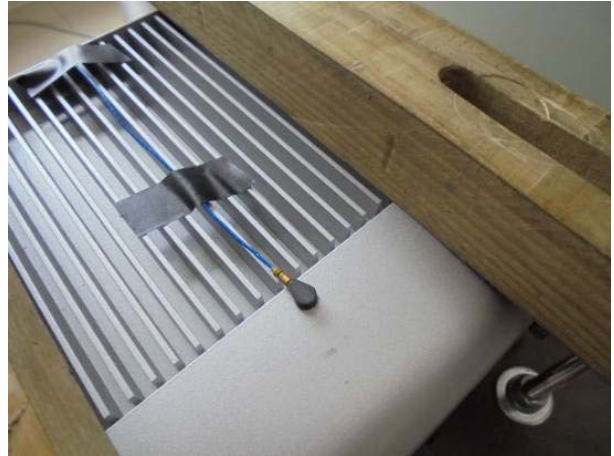
FIG.5.2 : Z Axis direction mounted.
