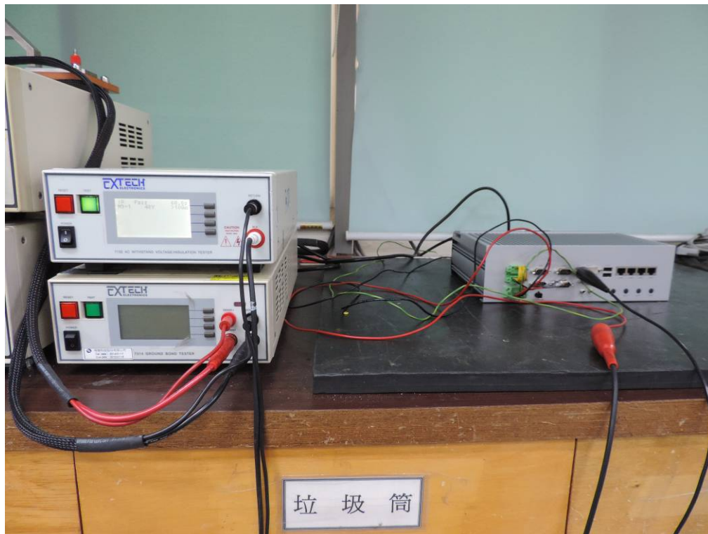
Insulation measurement Test (after high voltage test)
