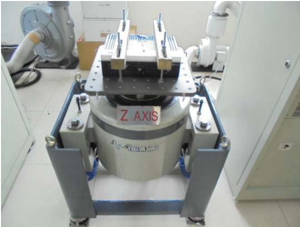
FIG.5.3 : Z Axis direction mounted.
