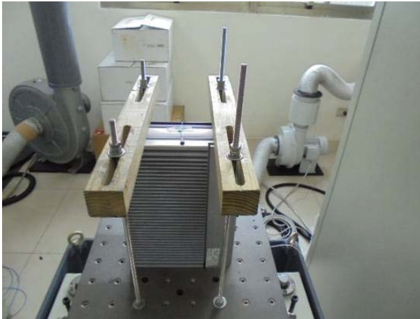
FIG.3.1 : Y Axis direction mounted.
