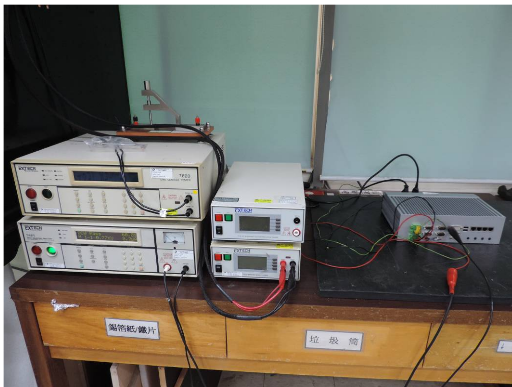
Voltage withstand test
