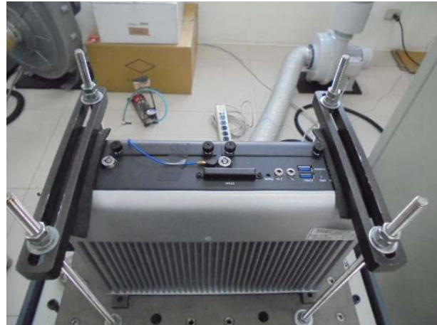
FIG.1.2 : X Axis direction mounted.
