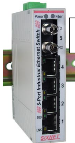
Typical ST style connector on a SL-5ES-2/3ST
