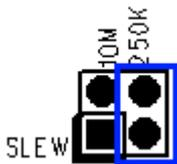
250K: Use Slew Rate Limit ability. Communication speed is limited under 250Kbps.
