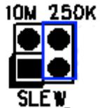
250K: Use Slew Rate Limit ability. Communication speed is limited under 250Kbps.
