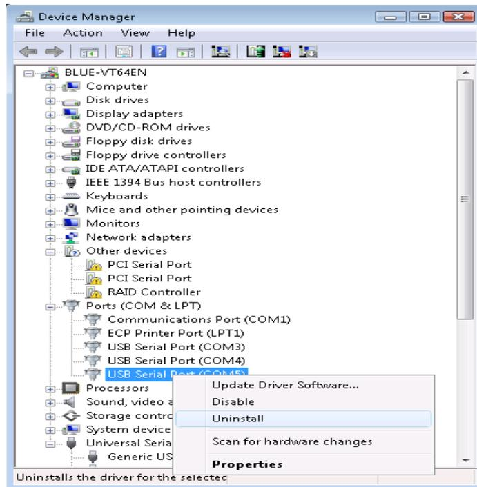
7. “USB Serial Port” removal is now completed. We will now continue with “USB Serial Converter” removal.
