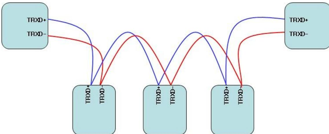
RS485, like LAN, uses Half Duplex Bus and has no classification between host and terminal.
