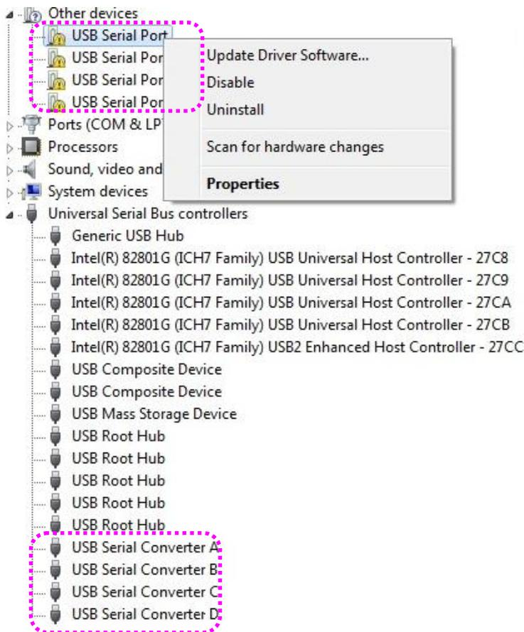
10. Following picture depicts “Device Manager” after carrying out all steps. As can be seen, all “USB Serial Converters” and “USB Serial Ports” are successfully installed.
