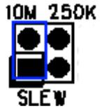
10M: Not use Slew Rate Limit ability. Maximum communication speed 921.6Kbps in this mode.
