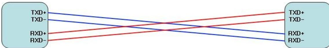
**- RS422 Multi-Drop Connection**
