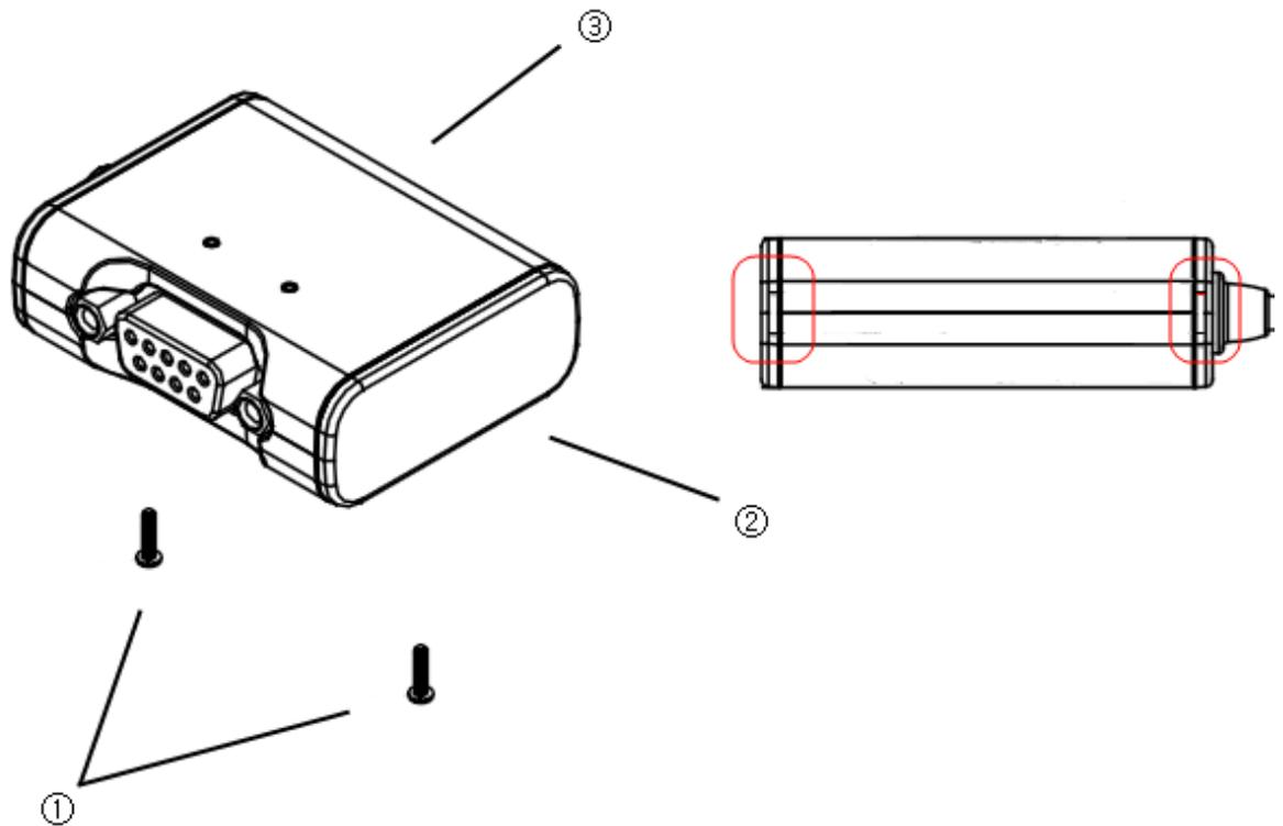
① Loosen the two screw on the bottom case.
