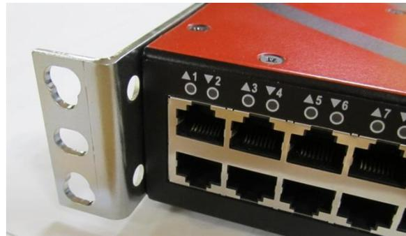
In the image above, the brackets are mounted so the front of the switch is setback 1/2 inch.
