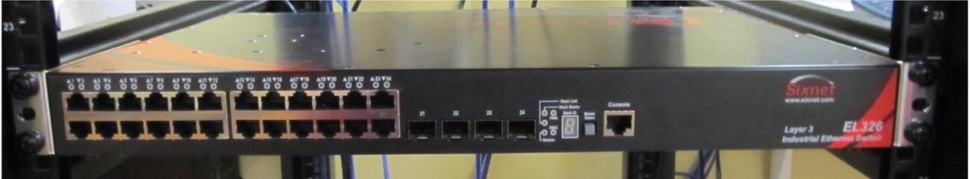
The above image shows an EL326 in front style arrangement (ports in front and power in the back) mounted in a typical 19" rack, prior to wiring.
