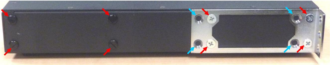
There are eight threaded inserts (see red arrows above) on each side of the switch that allow the brackets to be mounted in numerous positions for the best fit in your rack. The brackets also have extra holes (see blue arrows above) allowing them to be shifted right or left 1/2 inch. Use the supplied screws to mount the bracket in the desired position. Plastic screws are also provided to plug the unused holes. See below for possible mounting positions.
