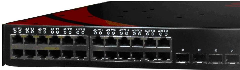
The RJ45 Ethernet port connector bodies on these products are metallic and are connected to the Chassis GND terminal. Therefore, shielded cables should be used to provide further protection from electrical noise and interference. Ideally, to prevent ground loops, the cable shield should be tied to the metal connector body at one end of the cable only. Electrical isolation is also provided on the Ethernet ports for increased reliability.
