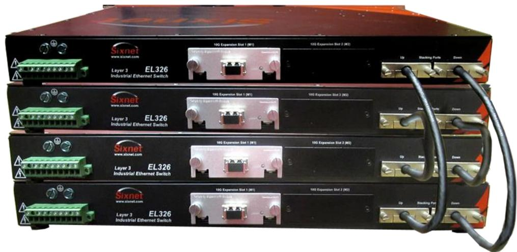
In line-topology stacking there is a single stack cable connection between each switch that carries two-way communications across the stack. In ring-topology stacking, an extra cable is connected between the top and bottom switches forming a "ring" or "closed-loop." The closed-loop cable provides a redundant path for the stack link, so if one link fails, stack communications can still be maintained.
