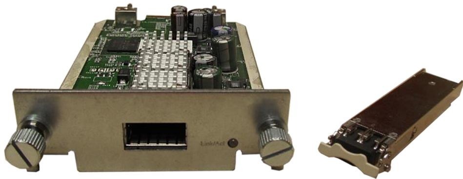
To install an optional 10G module into the switch, do the following:
