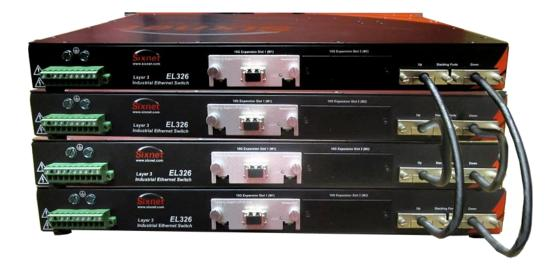
Connecting Switches in a Stack
