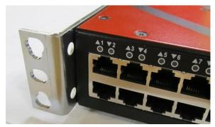
In the image above, the brackets are mounted so the front of the switch is setback 1/2 inch.
