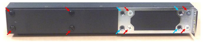
There are eight threaded inserts (see red arrows above) on each side of the switch that allow the brackets to be mounted in numerous positions for the best fit in your rack. The brackets also have extra holes (see blue arrows above) allowing them to be shifted right or left 1/2 inch. Use the supplied screws to mount the bracket in the desired position. Plastic screws are also provided to plug the unused holes. See below for possible mounting positions.
