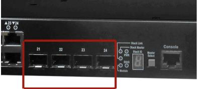
**Note:** For each of these ports you can only use one of the connectors (RJ45 or SFP) at a time. If you connect to both at the same time then neither connector may work.
