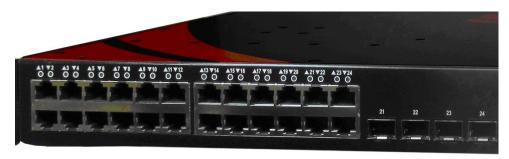
The RJ45 Ethernet port connector bodies on these products are metallic and are connected to the Chassis GND terminal. Therefore, shielded cables should be used to provide further protection from electrical noise and interference. Ideally, to prevent ground loops, the cable shield should be tied to the metal connector body at one end of the cable only. Electrical isolation is also provided on the Ethernet ports for increased reliability.
