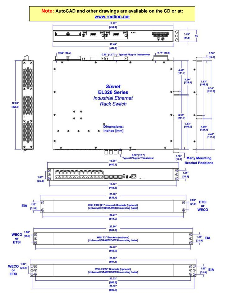
Mechanical Dimensions for the EL326 and Brackets
