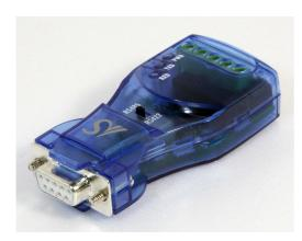
CS-428/9AT-ISO converts RS232 signals to RS422 or 485. It is an efficient solution for applying advantages of RS422/485 to legacy RS232 devices. The converter operates with no extra software installation, and with simple DIP switch toggling, RS422 or RS485 can be selected. CS-428/9AT-ISO has isolation protection so two electric circuits are completely isolated from each other. Also, the product is fully compatible with serial COM port in PC.
