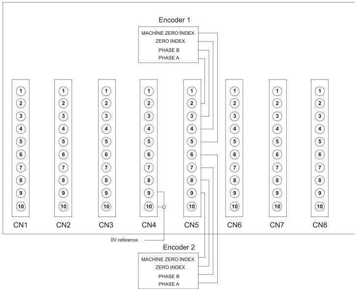
**Example:** Logic connection of two encoder modules. The encoder modules must be 24V powered (connect 0V reference of the encoder to the 0V of PLIO03 digital I/O supply)
