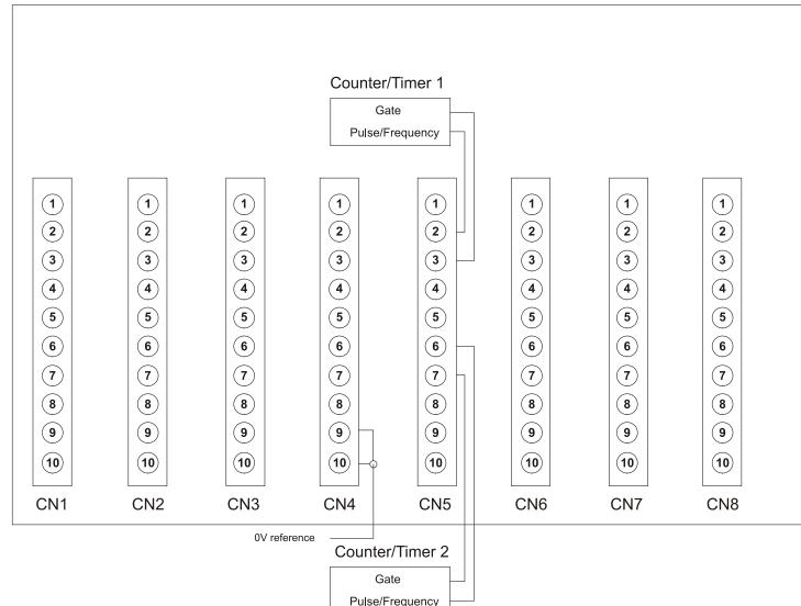
**Example:** Logic connection for two counter/timer measurement. Connection is suitable for counter inputs (pulse and gate) and/or frequency inputs (frequency and gate). The external modules must be 24V powered (connect 0V reference of the external module to the 0V of PLIO03 digital I/O supply)
