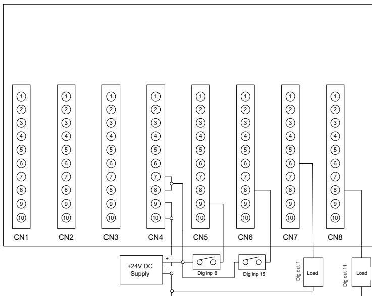
Example: Two digital inputs (switches) and two digital outputs connection.
