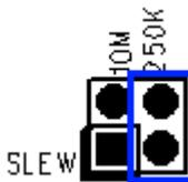
250K: Use Slew Rate Limit ability. Communication speed is limited under 250Kbps.
