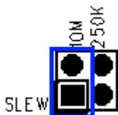
10M: Not use Slew Rate Limit ability. Maximum communication speed 921.6Kbps in this mode.
