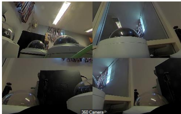
Optimum aspect ratio of the camera view with dewarp mode 'Quad view' is: any
