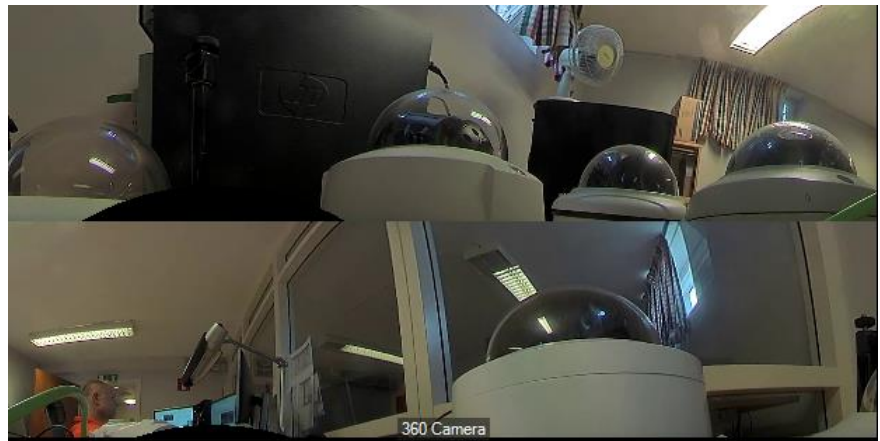
Optimum aspect ratio of the camera view with dewarp mode 'Double panorama view, fixed aspect' is: 2:1
