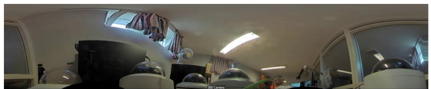
Optimum aspect ratio of the camera view with dewarp mode 'Panorama view' is: wider than 5:1
